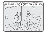
• Turn the J-dial counterclockwise. The still image moves back by one frame (one field).
